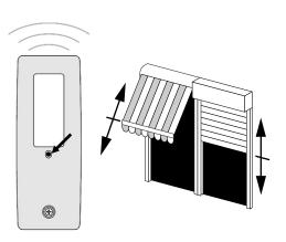
3) Touch the programming contact on the back of the Key Chain Transmitter with a metal conductor (paper clip). The LED on the front will start to flash
