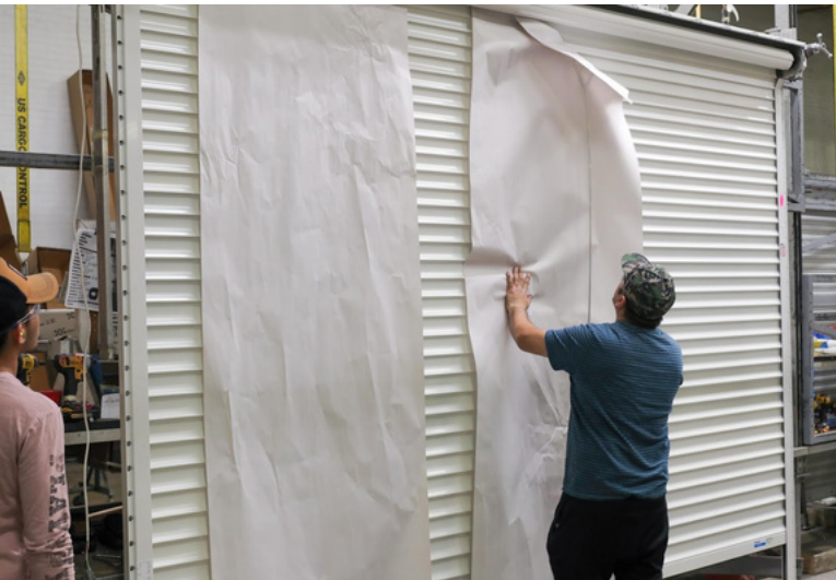
Before they reach your home, Qcompact shutters undergo rigorous operational run testing to ensure optimal performance and durability.
