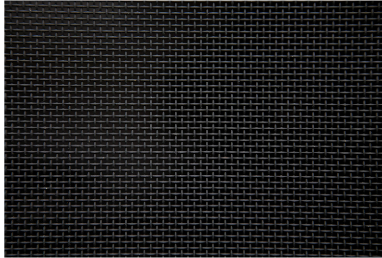
High-tensile 304-grade stainless steel mesh shown up close.
