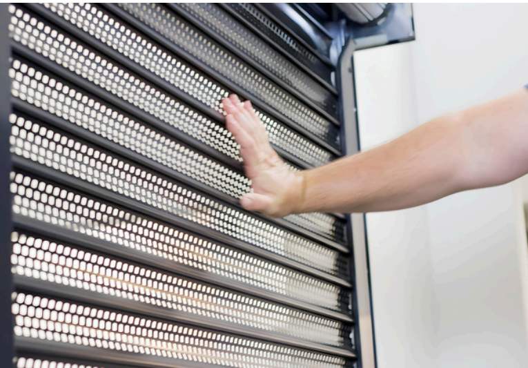
A perforated shutter curtain being tested for back-bend performance.
